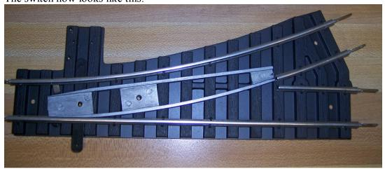
Next you will need to modify the base on the switch. A slot needs to be made between the elongated ties where the ground throw was just removed. The control linkage between the machine and the throw bar will pass through this slot. (The instructions with the switch motor indicate a ¼ hole is needed, we found that the hole needs to be elongated for linkage travel) \*\*\*\* See note at bottom of page
